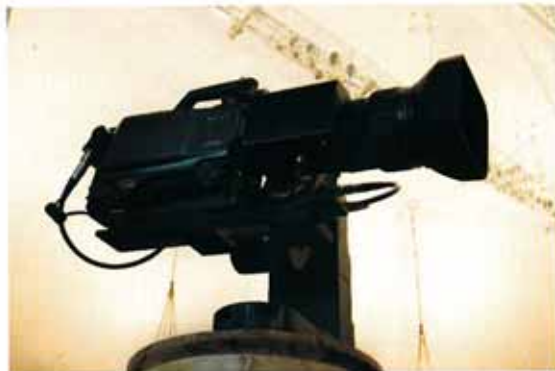
Right: For video capture, three Sony HDC1500L cameras are outfitted with Fujinon HA42X9.7BERD HD zoom lenses, using robotic control via Ravensclaw Talon remote camera heads for precise pan/tilt control.
